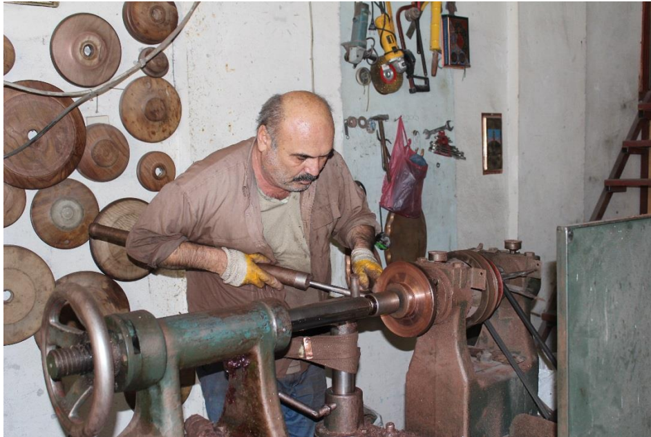
Photo 2. Shaping of a copper plate in spinning machine.
