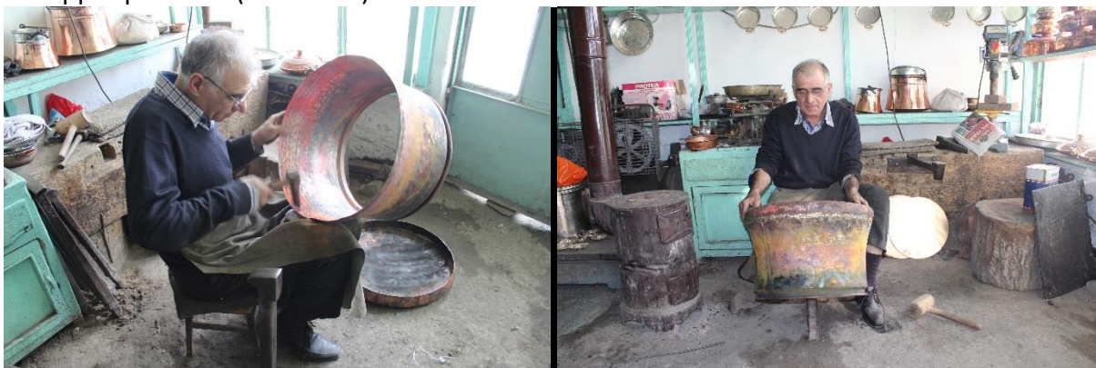
Photo 7. Making boiler with hammering technique
