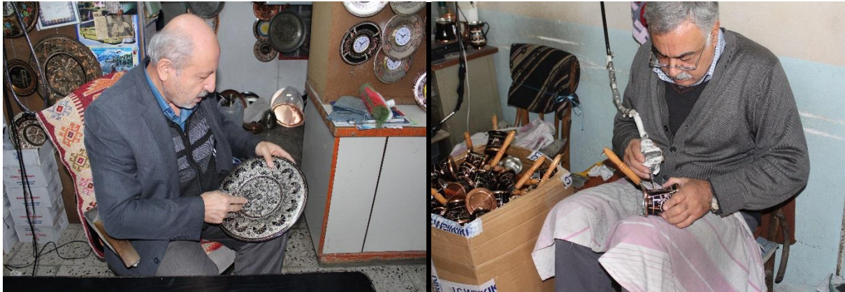
Photo 6. The processing phase of the copper products: Hand embroidery with pen (a) and machine hand embroidery (b).
