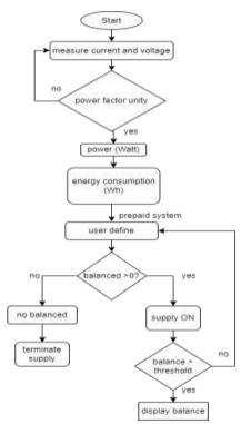
Figure 1: Flowchart for modeling single-phase prepaid energy meter using MATLAB/Simulink.
