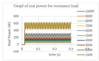
Figure 9: Varied active power between resistance of 100  $\Omega$  to 1000  $\Omega$
