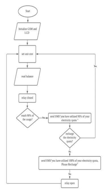
Figure 2: Flowchart for prototype single-phase prepaid energy meter
