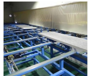
Figure 9: Longitudinal feed conveyor
