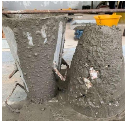
Figure 3: The result of the Slump Test
