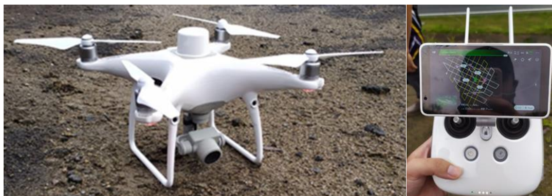
Figure 2. Drone and Flying Course for Mapping Area
