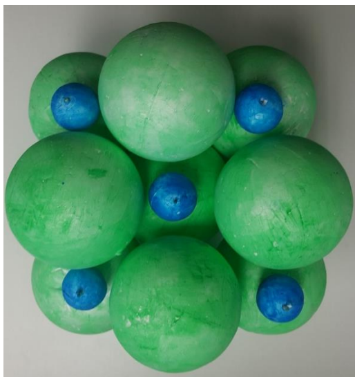
Figure 2. The crystal structure with face centre cubic (FCC) using the Ball and Stick model
