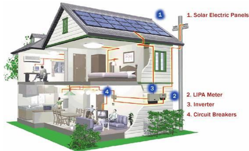
Figure 1. Solar system for residential
