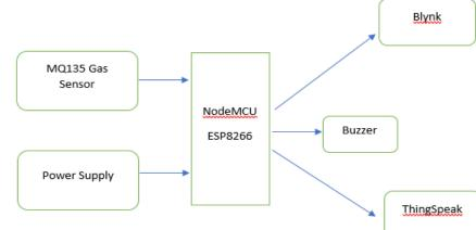
Figure 2: Block Diagram of Air Pollution Monitoring System
