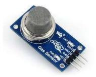
Figure 4: MQ135 Gas Sensor
