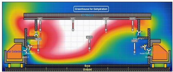
Figure 10: Simulation When Number of Heater Fan is One
