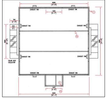
Figure 5: Top View Measurement Design of the Greenhouse
