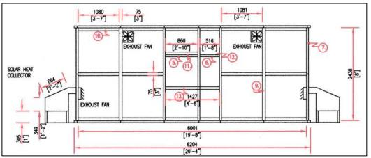
Figure 4: Side View Measurement Design of the Greenhouse
