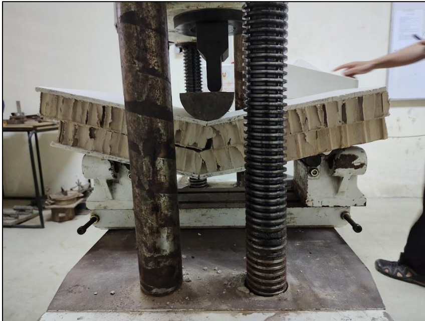
Fig. 9. Sample achieved maximum break force.
