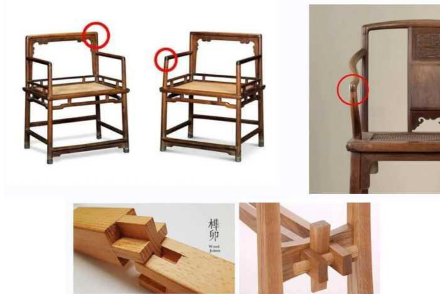
Figure 2. Ming furniture tenon structure (Flower Lai Sheng Ming, 2022)
