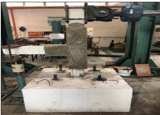
(k) Open Mould After 24 hours Apply R-ECC
