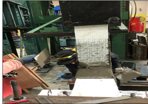
(h) Applied Base Lining with 10 mm of Thickness at The Sample
