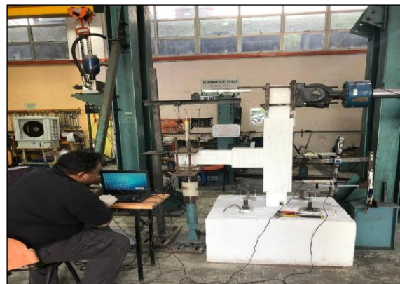
(l) Testing After Being Retrofitted for Sample 2
