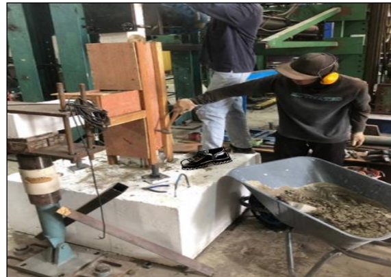
(j) Install Formwork and Fill RECC into Formwork with 20 mm of
