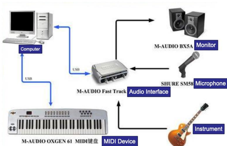
Figure 1: Digital audio equipment connection instructions diagram
