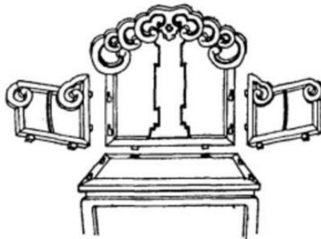
Figure 10: Mortise and Tenon Structure of Cantonese-Style Chair
