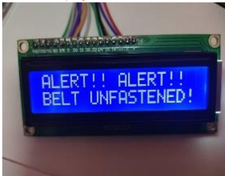
Fig.9 LCD shows status when the seat belt is unfastened
