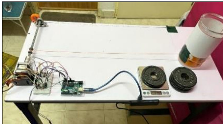
Figure 4: Bipolar NEMA17 Stepper Motor with Load Setup
