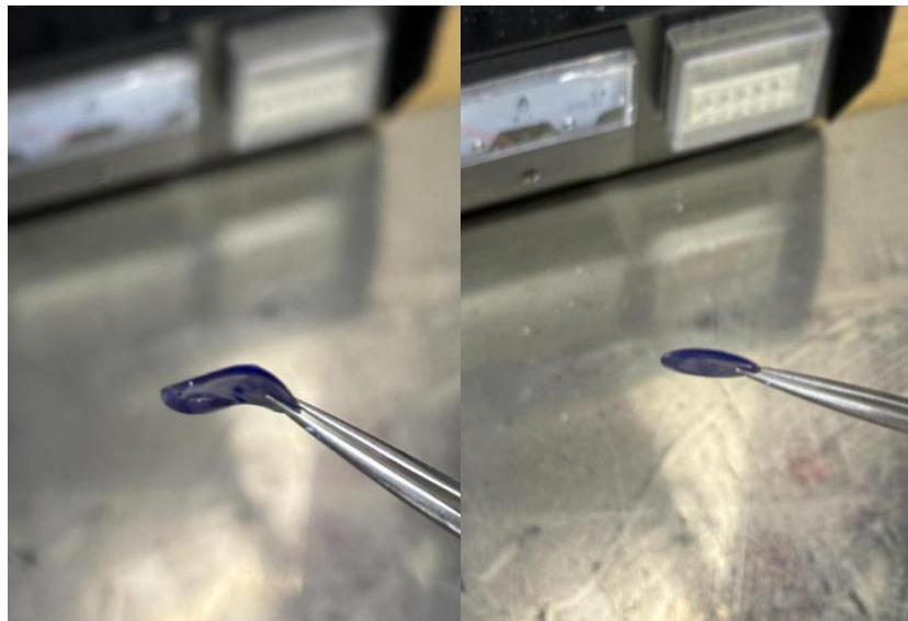
(Figure11) The image on the left is Deformation Degree of 0.2 mm Purple Copper Sample Fired at 750°C. Image source: Photographed by the author.
